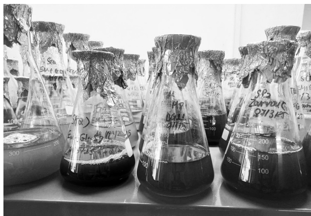
Figure 2. Inoculum cultivation of S. salina M8 in a 250 mL Erlenmeyer flask
